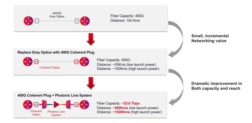
Coherent optics works the photonic line system to maximize fiber capacity and performance
