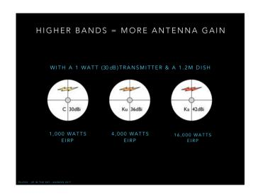
And the converse of antenna size is gain. Here we use the same size dish at the three different bands.
