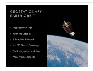
Geostationary orbit is around 36,000 km away from Earth.
