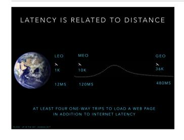
This view is roughly to scale, and I've put the curve where it belongs. And here's our first three things - orbital levels. Low Earth, Medium Earth, and Geostationary Orbits.
