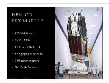
We're looking at the second NBNCo Sky Muster satellite, and I left some engineers in for scale. This one project is putting 135 gbps of capacity in the skies over Australia. It's Ka band, which means it will have rain fade issues, but for the most part its remote users are in places it doesn't rain a lot. Still at least 430 ms latency from its GEO orbit, but heaps faster than New Zealand's farmside service.
